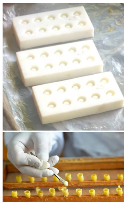
Figure 1. Silicone molds for casting wax bowls and wax bowls
