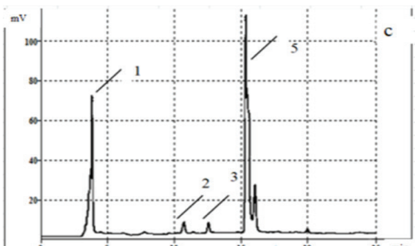
Figure 1. HPLC analysis of oat bran polyphenols obtained using physical (a), chemical (b) and enzymatic hydrolysis (c) extraction methods: 1 - gallic, 2 - 4-hydroxybenzoic, 3 - chlorogenic, 4 - p-coumaric, 5 - ferulic acids
