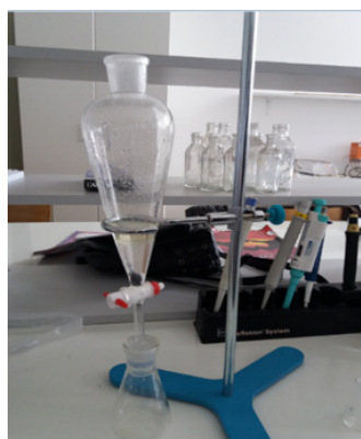
Figure 3. Extraction technique in obtaining black cumin extract
