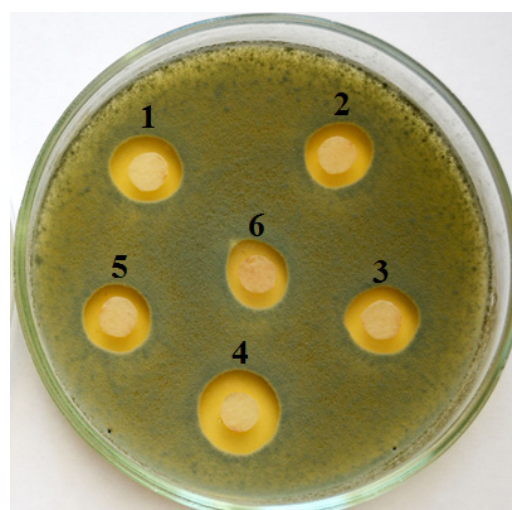
Figure 3. Photo of a Petri dish with mold culture Penicillium roqueforti with discs impregnated by nanosilver samples of stabilized with DDAB, with different values of the active acidity of the medium (pH): 1. pH = 3; 2. pH = 5; 3. pH = 6; 4. pH = 8; 5. pH = 9; 6. pH = 11
