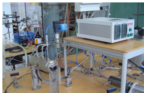
Figure 2. High pressure view cell: flow sheet (a) and photo (b) of the apparatus
