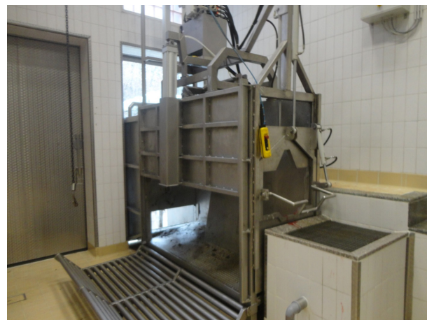
Figure 3. Box for halal slaughter with a tub for blood draining
