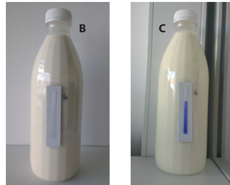
Figure 5. The chromogenic temperature indicator on packaging of milk: activated at room temperature (B) and activated after putting it again at refrigeration temperature (C)
