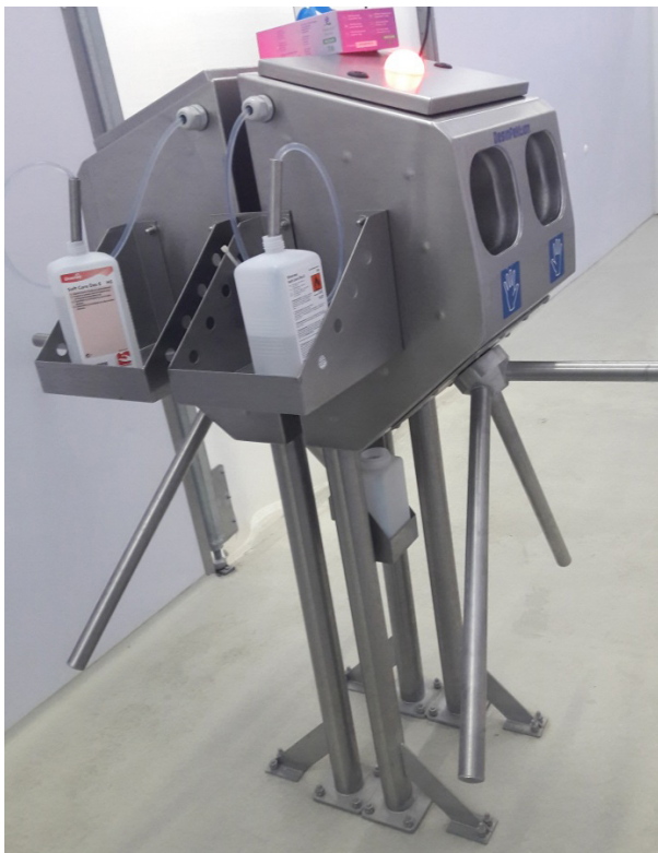
Figure 2. Hand disinfection station in final snails meat processing facilities
