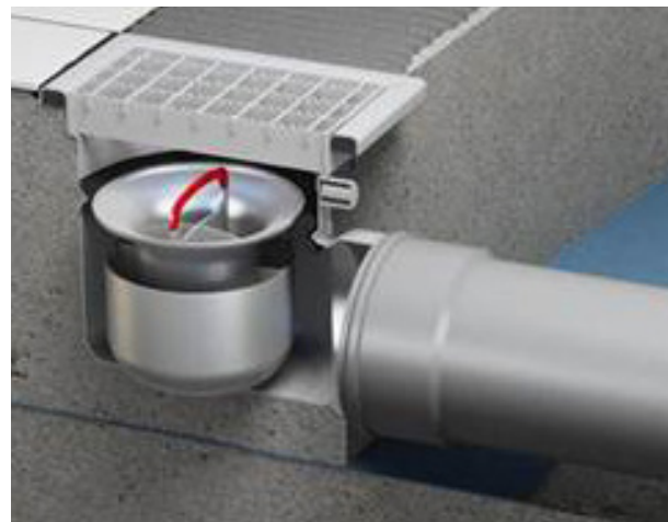
Figure 3. Gully with removable foul air trap with connection to on-going drainage and sewer
