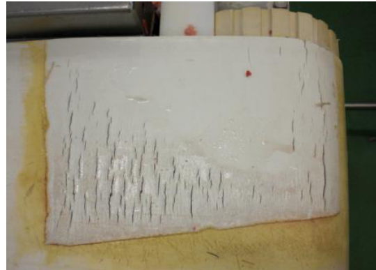
Figure 4. Cracks and crevices on the belt surface
