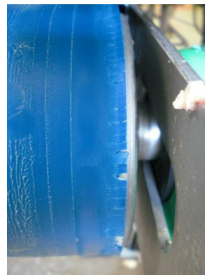
Figure 5. Cracks and crevices on the belt edge
