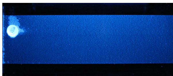
Figure 2. Original protein film on stainless steel surface. UV-illumination (wavelength 312 nm). Dark areas: clean areas; lighter color: soiled areas.
