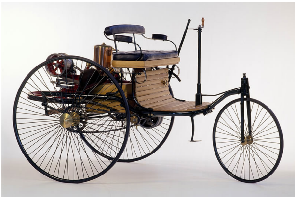
Figure 4. Even one of the first patented cars in 1886 by Benz is a transformational change based on existing horse carts, bicycles, and relatively a new development, a gasoline engine visibly brought together [15]
